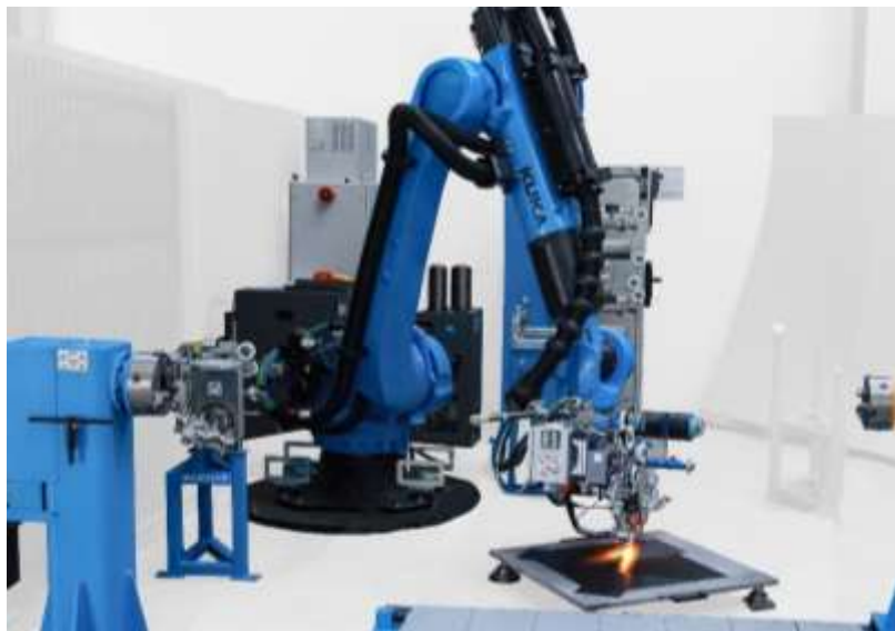
Single Tape Placement and Robotic Filament Winding Equipment at Mikrosam
