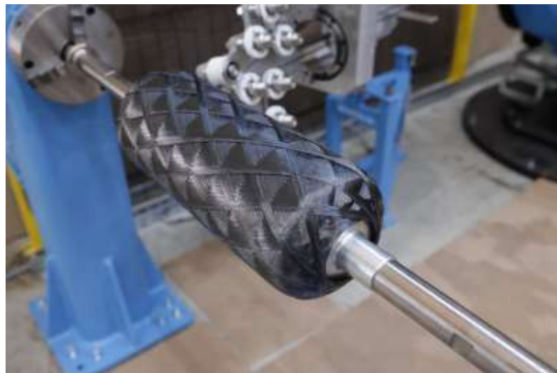
Robotic towpreg winding process
